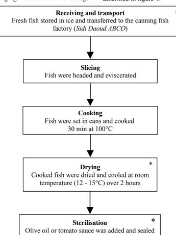
Figure 1: Flow diagram of the production of *Sardinella aurita* and *Sardina pilchardus* cans. \* correspond to tissue sampling (n= 9 in each time) at different processing
